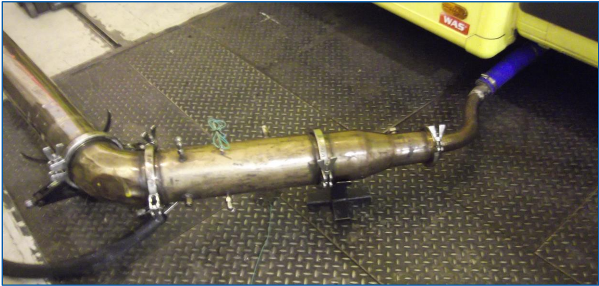
Figure 8 - Emissions sampling equipment connection to vehicle
