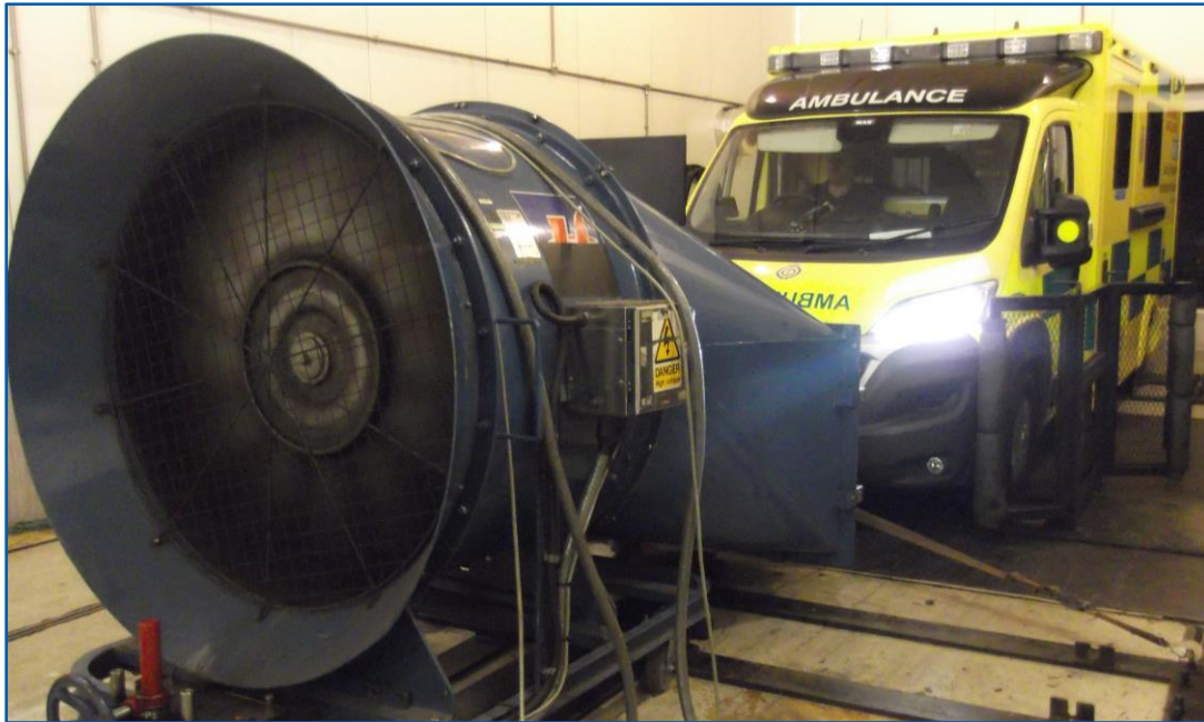
Figure 10 - Test vehicle on chassis dynamometer during testing in the VTEC
