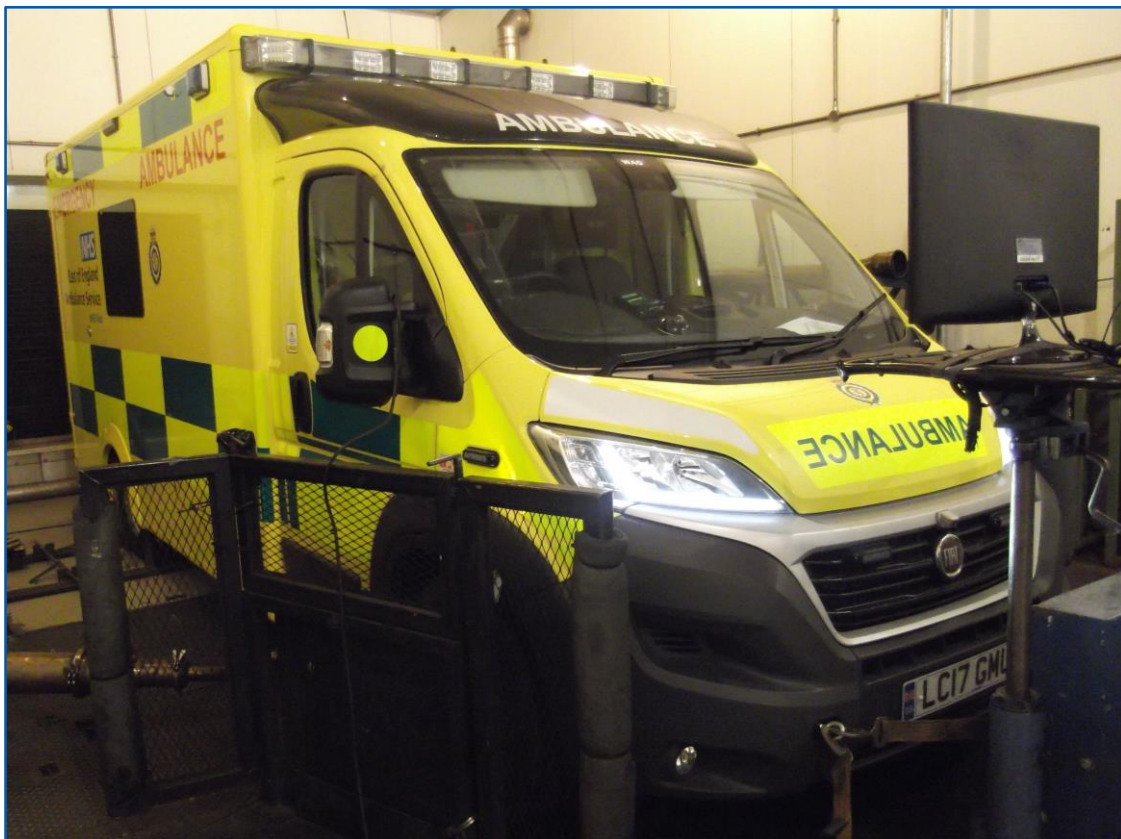
Figure 11 - Test vehicle on chassis dynamometer during testing in the VTEC
