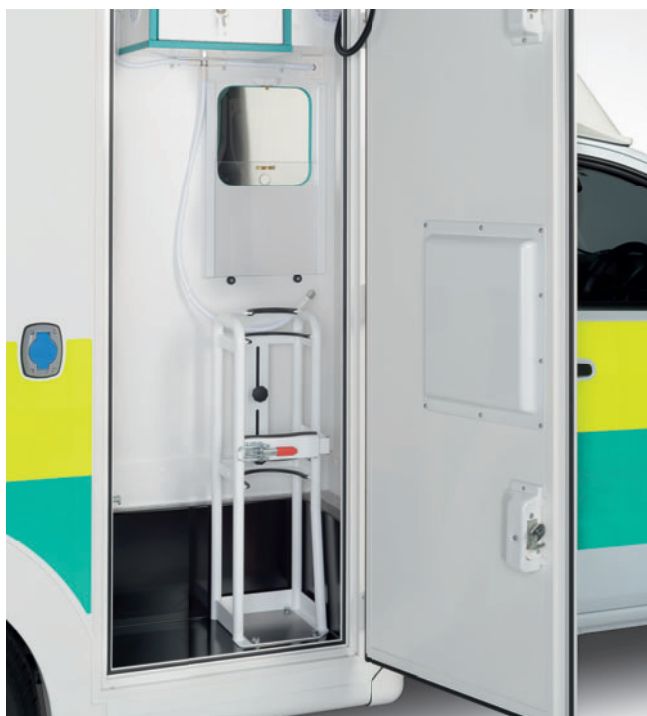
External access to medical gas storage compartment.
