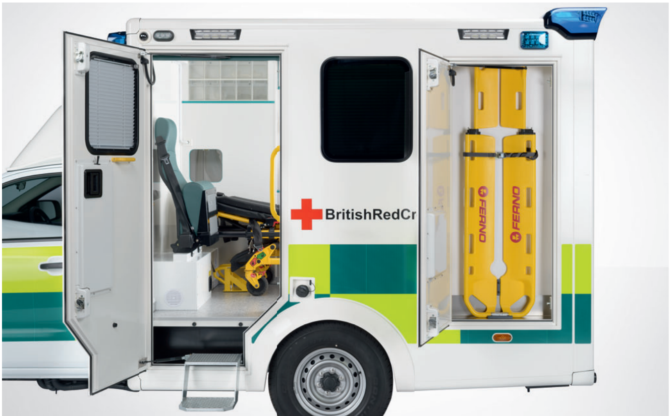
Full size saloon access door with auto deploy side step and rear external locker for scoop stretcher.
