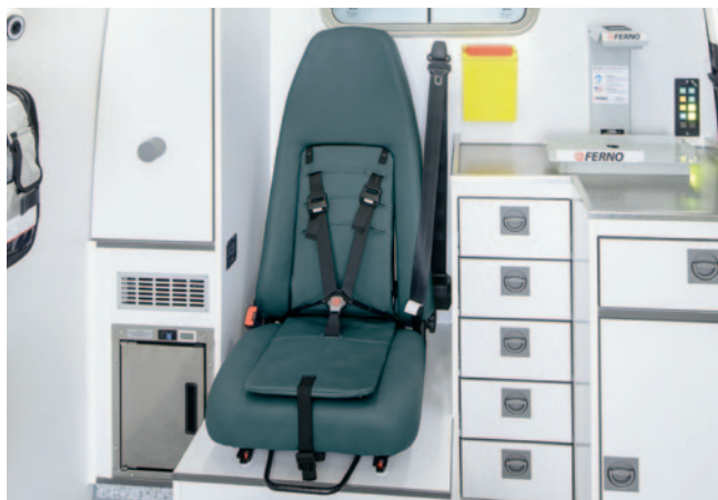
Doctor's seat with forward and backward movement. An additional ISOFIX child restraint seat with 4 point child's seat belt is integrated.
