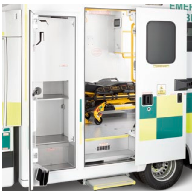
The external access hatches ensure time-saving removal of equipment.
