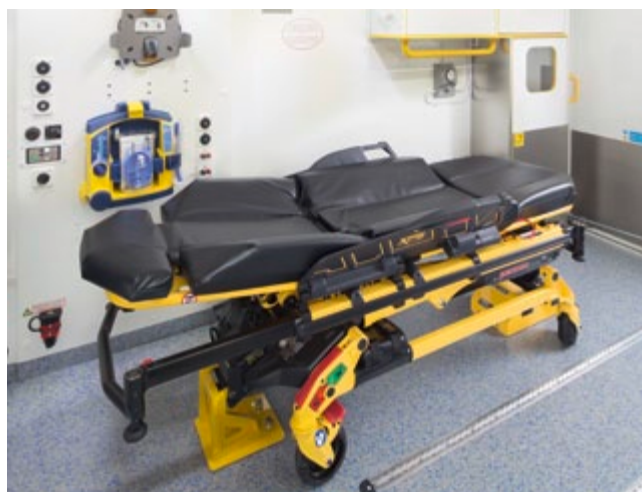
Airline rails in the floor facilitate multiple options for mounting a standard or a bariatric stretcher.
