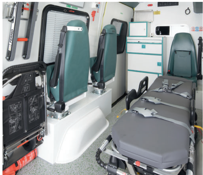
Medical attendants seats can easily be rotated and folded away.
